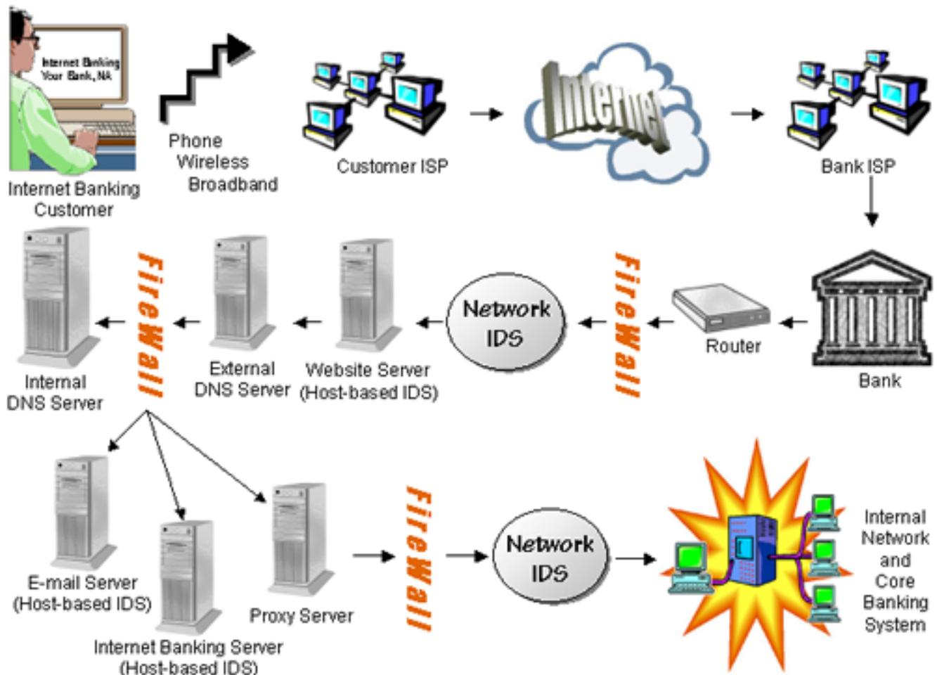
**Text Description of Figure 2** This diagram illustrates the transaction flow for one possible configuration in which the bank hosts the Internet banking application.
